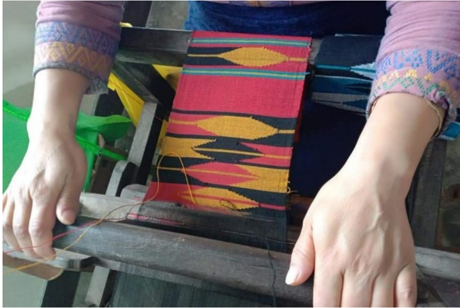
Wooden loom with warp and weft
